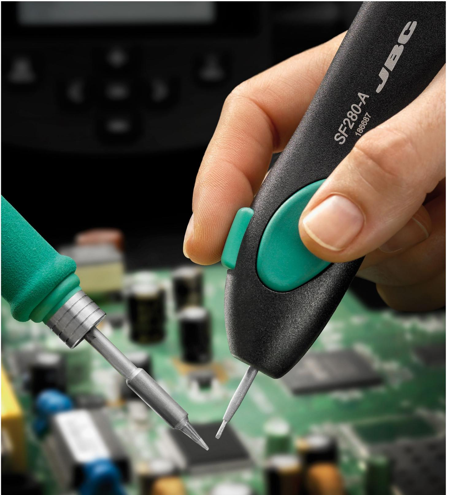
**Automatic** Solder Feeder V-Cut
